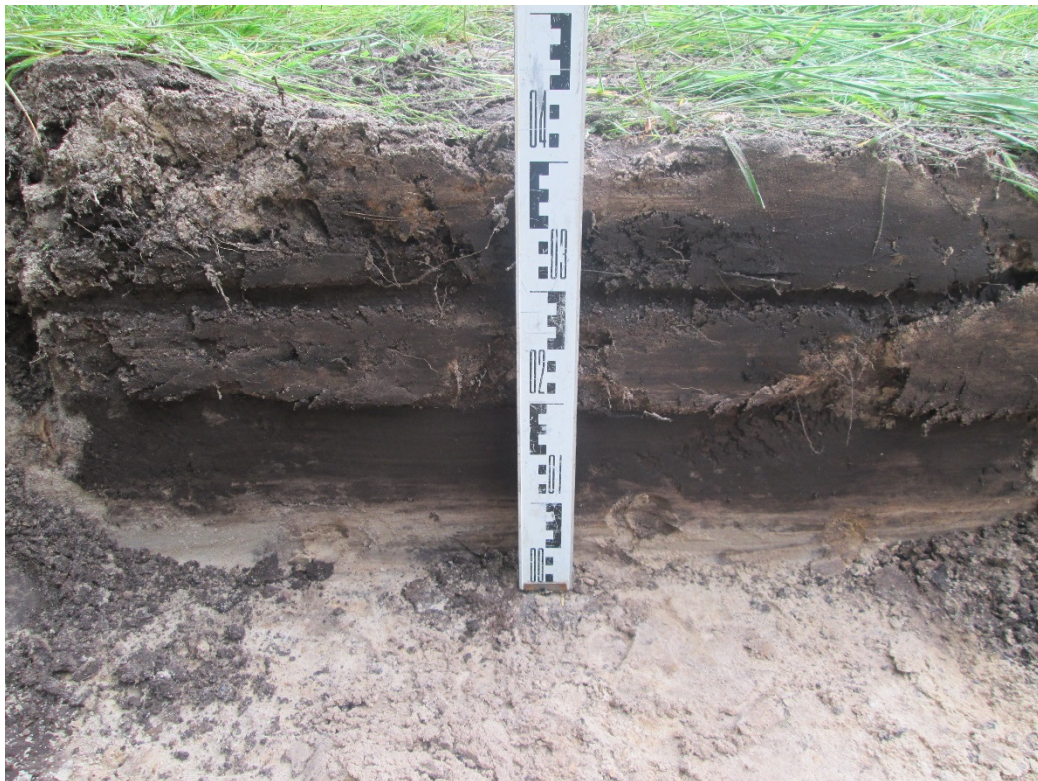
Diepte bepaling putbodem / putwand
